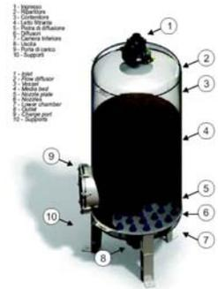
The FQR Filter Vessels are carbon steel tanks with protection of surfaces by galvanizing or thermal polyurethane coating (enamel on request). A strong nozzle plate, equipped nozzles per m<sup>2</sup>, allows the vessel for filtration process by:
