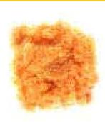
D42 MACROPOROUS POLYSTYRENE CHELATING RESIN 1.0 Applicable Standard of Product: Q/320281, NAN06-1997 2.0 Indexes of Physical and Chemical Properties: Characteristics
