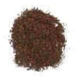
ودعري CSG-OXYPURE Manganese Dioxide Iron, Manganese, Hydrogen Sulfide, Reduction Media - 20 x 40 Mesh Batch.No.220208 14,5 L ( 1/2 Cu.FT) Handling and storage instructions Net weight 20 Kg
