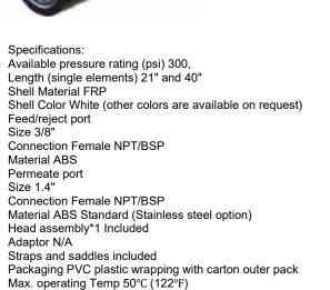
Note: \*1- Head assembly consists of halfmoon lock plates, ABS seal plate and lock nut, Head seal, permeate port o-ring. (cast Aluminum bearing plate only used in 1000 psi vessel)
