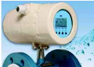
Measuring stub pipe with nominal diameter from 15 to 1600mm.Measuring range: 0-10 m/s Accuracy: +/- 0,2% of measured value with velocity of the fluid >0,2m/s. Materials: Internal tube: stainless steel AISI304; Connecting flange: carbon steel; Internal lining:PTFE for diameter > DN 100 in food compliant ebonite. Electrodes: Hastelloy C (Titanium, Tantalum or platinum upon request) Housing protection: IP67 (compact) –(on request IP68 - only for remote versions sensor ).
