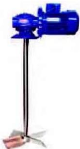
Slow mixers are used in water treatment plants. The shaft of the mixer is directly key coupled with the hollow of the Worm gear box, supplied with shaft and impeller 4 blades 45°. Single phase motor (available up to 0.37kW); +5% pH motors, upon request 1-pH motors for power supply lower than 0.37 kW (+5%). Materials SS 304 (standard) - AISI 316 +8%, shaft and impeller sheathed in Rubber Ebanite (upon request) or PVC +25%, shaft and impeller in PP covering a steel core (+30%).
