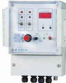
Controller designed to measure, control and regulate the pH value • Measuring range 0÷14 pH. • Temperature compensation • Numeric LCD (3 digits) • Regulation of 2 independent intervention set-points • 2 ON/OFF outputs • Output 4-20 mA • Power consumption 6 Watts • Electrode supplied upon request
