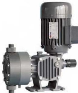
flow rates up to 116 l/h (30,64 US Gal/h), at 50 Hz, 139 l/h (36,76 US Gal/h) at 60 Hz, pressure up to 16 bar (232 psi) at 50 Hz and 60 Hz phase 60 Hz isolation class F
