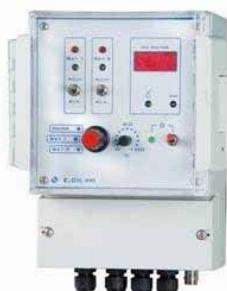
Controller designed to measure, control and regulate the free residual Chlorine value • Measuring range 0÷10 ppm • Numeric LCD (3 digits) • Regulation of 2 independent intervention set points • 2 ON/OFF outputs • Output 4 - 20 mA • Power consumption 2 Watts • Chlorine Cell supplied upon request
