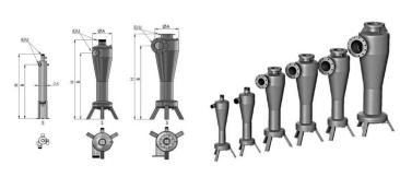
The hydrocyclone filter, or filter ring, or centrifugal separator sand, is often considered a pre-filter for the cleaning of liquids or very sandy or saturated
